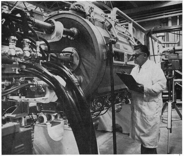
EXTREMELY HIGH TEMPERATURES and high velocities are simulated in the test chamber of one-megawatt plasma generator located in Aerophysics Section
